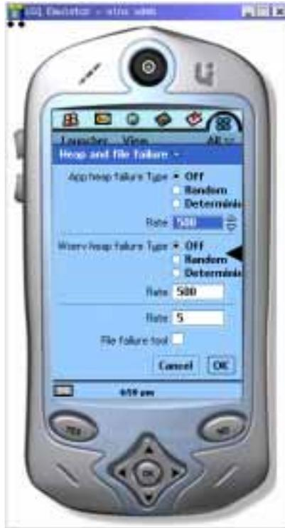
Using the Uikon debug key sequence Ctrl+Alt+Shift+P, the tool comes up, allowing one to set deterministic or random failure points for both fileserver resources and memory allocations. Note that such treatment, from the tool, applies only to the application context from which it was called.
